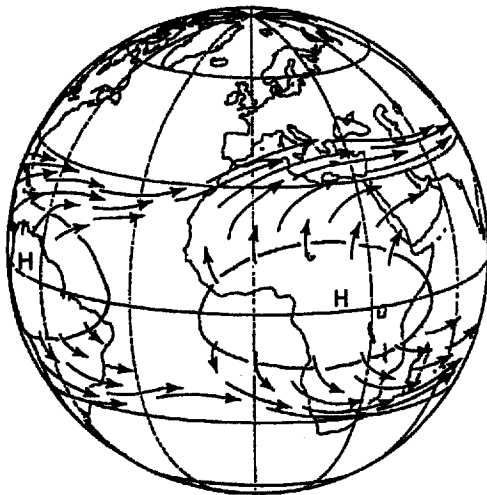
Figure 15 A schematic illustration of the formation of the subtropical jet stream. Air accelerated by the upper-tropospheric PGF gains speed poleward, but is simultaneously affected by the fV , which, by deflecting it clockwise in the Northern Hemisphere (anti-clockwise in the Southern Hemisphere) tries to bring the air back towards the equator. A balance is reached around 30^\circ latitude
