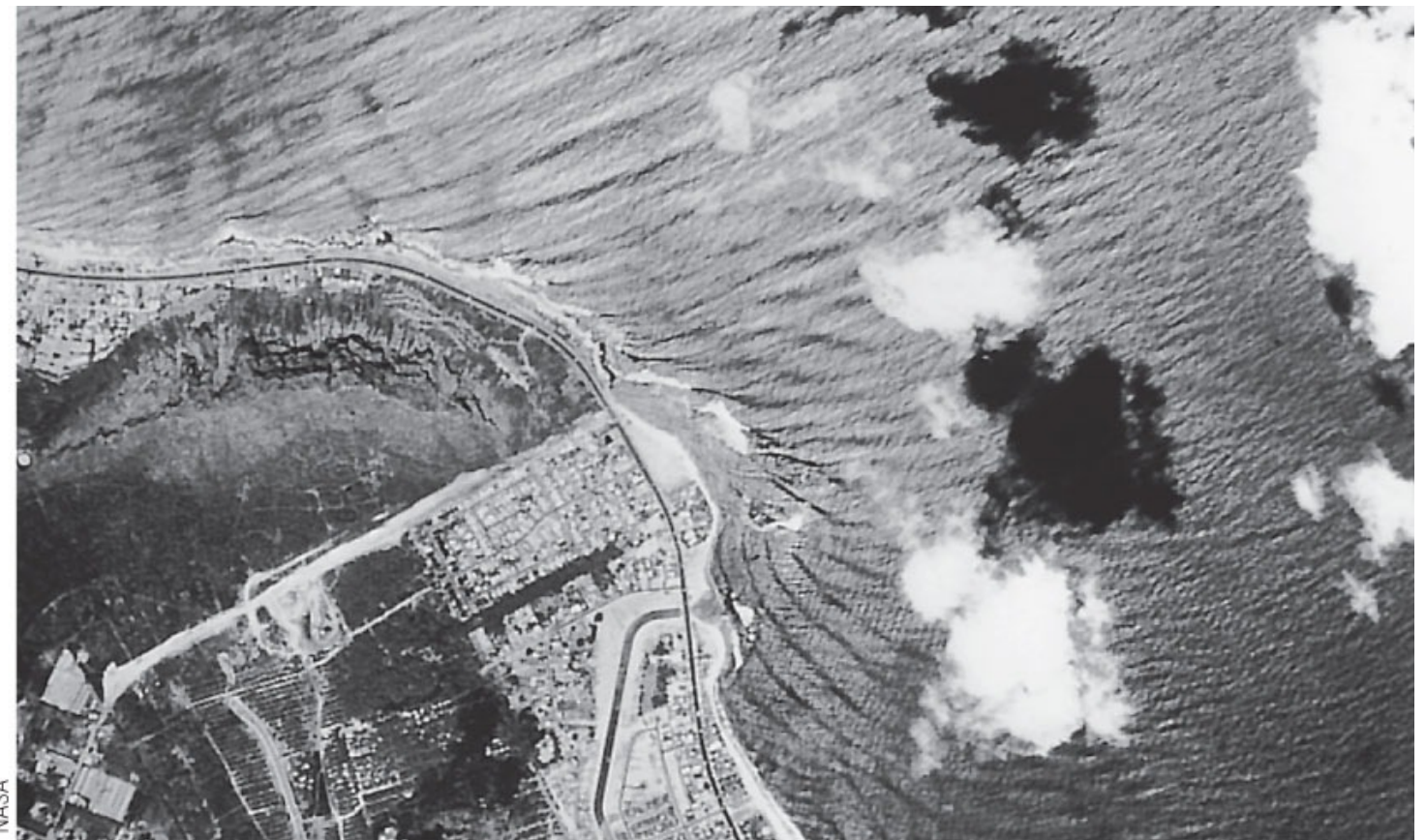
b Wave refraction around Maili Point, O'ahu, Hawai'i. Note how the wave crests bend almost 90^\circ as they move around the point.
